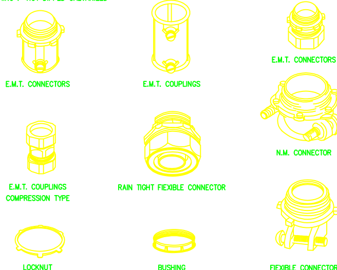
05 TYPICAL DETAIL FOR CONDUIT FITTING NTS
