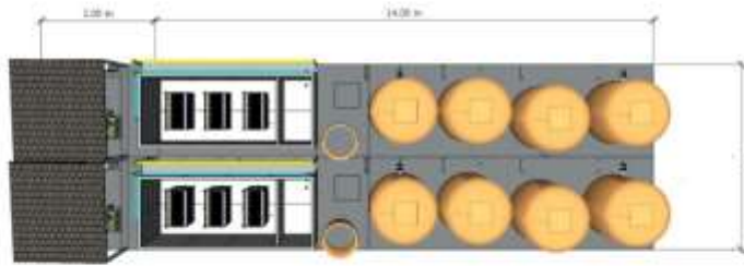
Horizontal Bio-Reactor (MSR) Westwater Treatment Plant Effluent BOD 150.00 mg/L Effluent BOD 150 mg/L, Effluent BOD = 30 mg/L.
